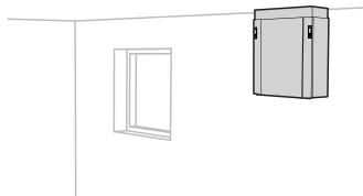
Suspended from the ceiling . A ceiling mounting must be fitted (available as an accessory).
